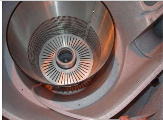
11) Connect the new back wash air tube to the other side of the air valve.
