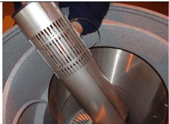
13) Position the supplied Jubilee Clip (band clamp) at the base of the centre pipe and tighten fully.
